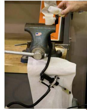
1.5 Check that the tank is full. Tilt the end of the reservoir of M / C again until a nearly vertical position (the end of the rod pointing down). Slowly and steadily push the stem into the M / C until it feels substantial resistance. Repeat this several times. Observe the tank to see that no air coming out of the M / C. Continue doing this until the stem only 2 mm displacement required before feeling the increased load.
