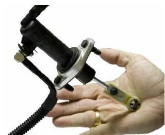
1.7 If the system complies with the 2 mm verified, then check that the rod strap S / C is in place so as to maintain the stem of S / C in their particular position.
